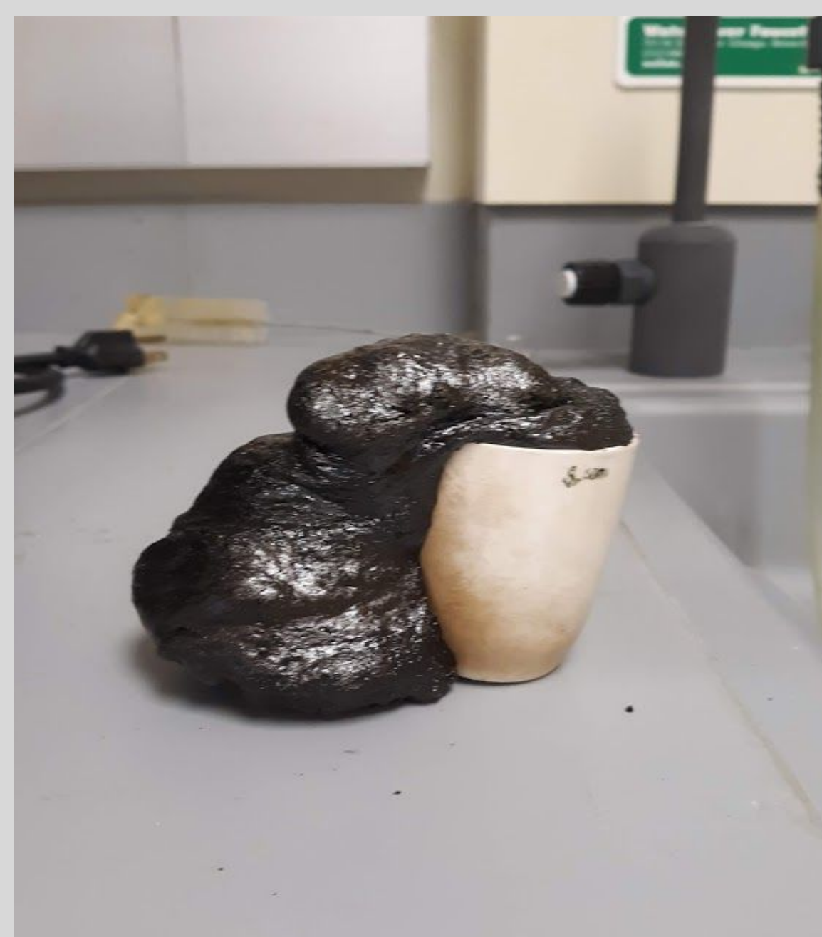
Figure 2. Honey sample 2 exploded in the muffle furnace during the dry ashing process due to residual moisture.
