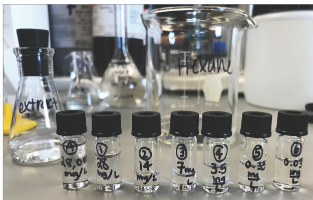
Figure 4. Six standards created through a serial dilution. The original hexane extract (far left vial) was created through the Fischer esterification procedure. Source: Katharine Colley.
