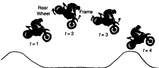
Fig. 4. To correct "endoing," the rider can accelerate rotation of the rear wheel to lift the front wheel for a safe landing. At  $t = 1$ , the rear wheel has begun to drop too low for a safe landing. At  $t = 2$ , the rider is accelerating the rear wheel, which begins to rotate the frame upwards. At  $t = 3$ , the frame is continuing upward rotation until a safe position is achieved at  $t = 4$ .
