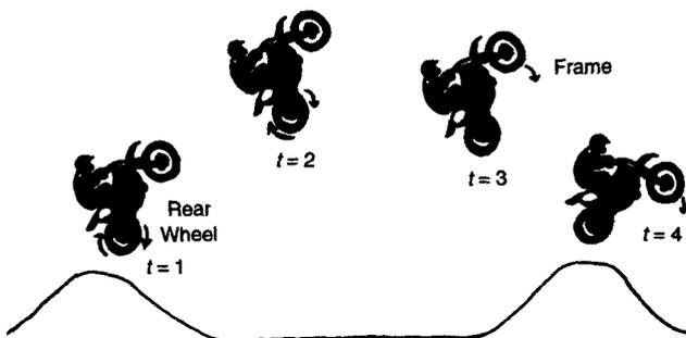
Fig. 3. To correct "looping out," the rider can stop rotation of the rear wheel to bring the motorcycle to a more stable position. At  $t = 1$ , the rider has just left the ramp and the front wheel is beginning to lift too high. The front wheel is too high for a safe landing at  $t = 2$ . At  $t = 3$ , the rider has locked the rear wheel and the motorcycle frame is beginning to rotate downward. At  $t = 4$ , the frame is continuing to rotate downward for a safe landing.
