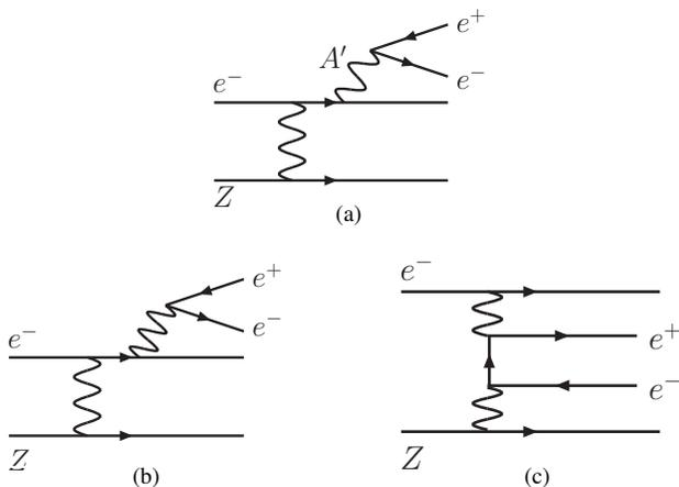
FIG. 1. *Top*: (a)  $A'$  production from radiation off an incoming  $e^-$  beam incident on a target consisting of nuclei of atomic number  $Z$ . APEX is sensitive to  $A'$  decays to  $e^+e^-$  pairs, although decays to  $\mu^+\mu^-$  pairs are possible for  $A'$  masses  $m_{A'} > 2m_\mu$ . *Bottom*: QED trident backgrounds: (b) *radiative* tridents and (c) *Bethe-Heitler* tridents.
