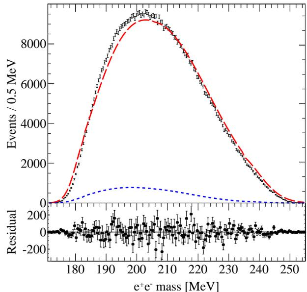
FIG. 3. *Upper panel:* The invariant mass spectrum of  $e^+e^-$  pair events in the final event sample (black points, with error bars), accidental  $e^+e^-$  coincidence events (blue short-dash line), and the QED calculation of the trident background added to the accidental event sample (red long-dash line). *Lower panel:* the bin-by-bin residuals with respect to a 10-parameter fit to the global distribution (for illustration only, not used in the analysis).
